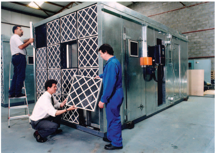
IAC acoustic AHU during assembly
