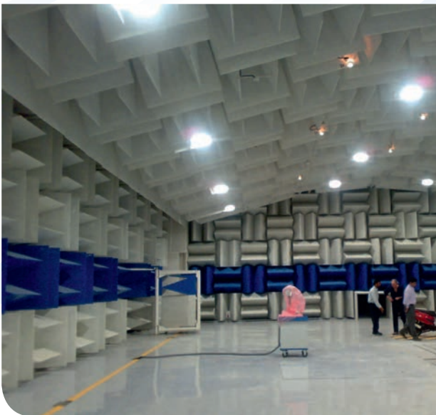
Hemi-anechoic pass-by chamber for Bajaj Motorcycles, India
